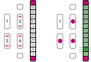
**Sensor is ready for operation (measuring mode)**
